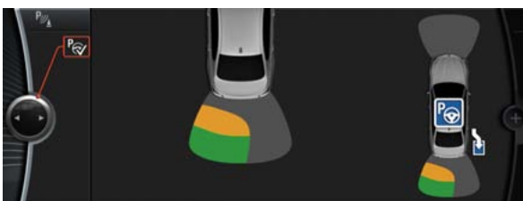
F10 parking assistant, parking display during the parking process
